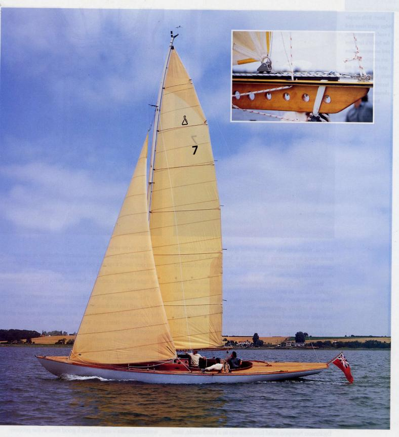
The keel carries a flattened bulb for maximum effect and o encourage the high/low pressure separation of waterow across the keel. Both keel and rudder have vortex tips o reduce turbulence and an end plate reduces the rudder's endency to stall at very high or low speeds.
